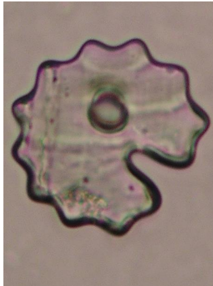
Figure 7: “Chickenhead” taggant with PVOH component removed
