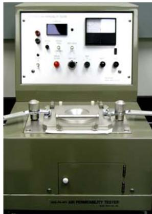
**Figure 3.10.** KLS Airflow Resistivity Tester
